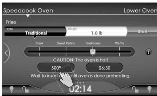
2. Tap the displayed temperature (500° in the screen shown above). The temperature bar will display.
