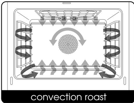
Convection Roast uses the same heating elements as Roast. However, unlike Roast, Convection Roast utilizes the convection fan and heater in the back of the oven to help heat and circulate the air throughout the cook cavity.
