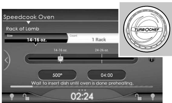
The LED light ring, beside the touch screen, is also synced with the progress meter to show preheat status.
