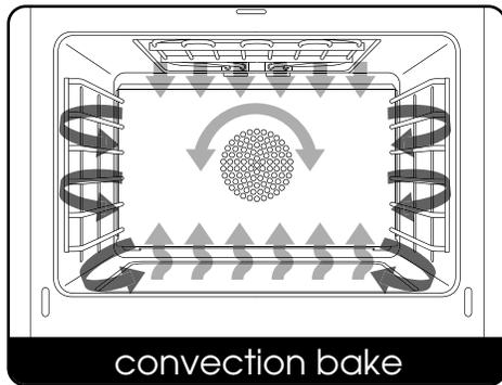
Convection Bake uses the same heating elements as Bake, with the addition of a convection fan and heater in the back of the cook cavity. This fan and heater help heat and circulate the air evenly throughout the chamber to produce superior browning and crisping.
