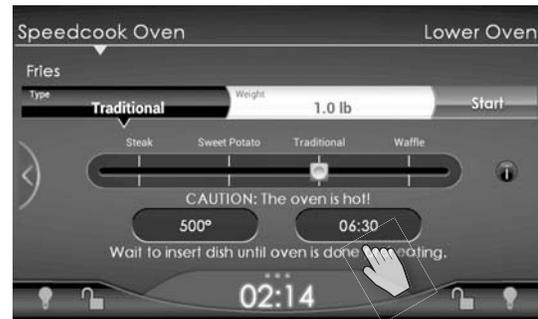
2. Tap the displayed time (**06:30** on this screen). A keypad will display, allowing you to enter a new time.
