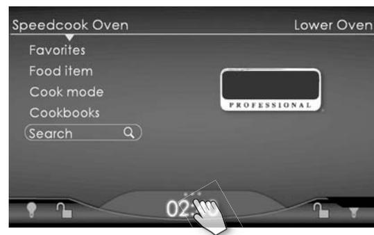
For access to the utilities, including the clock, and the timer, tap the three dots above the clock time on the tab in the middle of the bottom of the screen. The tab will pull up, showing two sections, one for utilities and one for the timer, as shown below:
