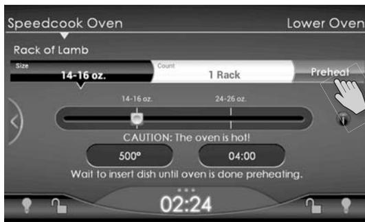
2. Preheat progress is displayed on the status bar and LED light ring. Preheating will take 8-14 minutes. The oven will chime when preheating is complete. The preheating progress will be displayed on a bar near the bottom of the screen.
