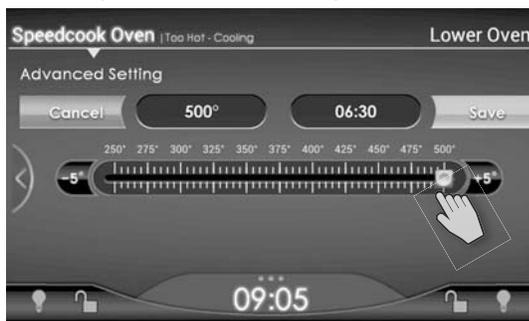
3. Drag the button (which moves in 5° F increments) to the new temperature.
