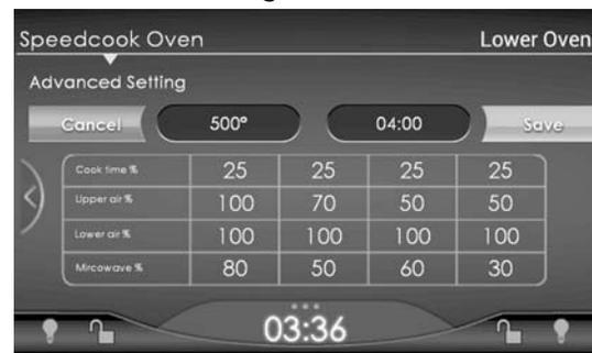
5. Make any adjustments you wish to make to upper air intensity, lower air intensity, or microwave power.
