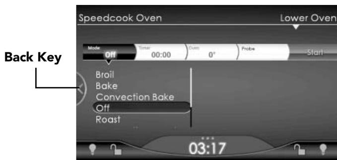
2. To go from the Speedcook Oven to a Lower Oven screen, tap **Lower Oven**.
