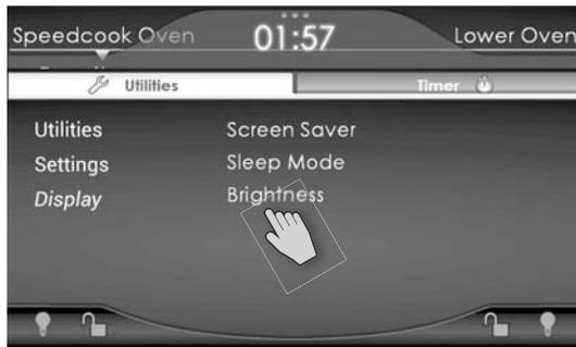
2. To adjust brightness select **Brightness**. The screen displays the brightness bar, which allows you to change the display brightness from low (on the left) to high
