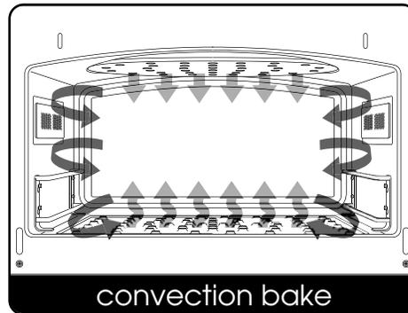
When set to Convection Bake, the Speedcook Oven operates as a standard convection oven with the fans running at a low speed. This function creates the same cooking environment as the Lower Oven in Convection Bake mode.
