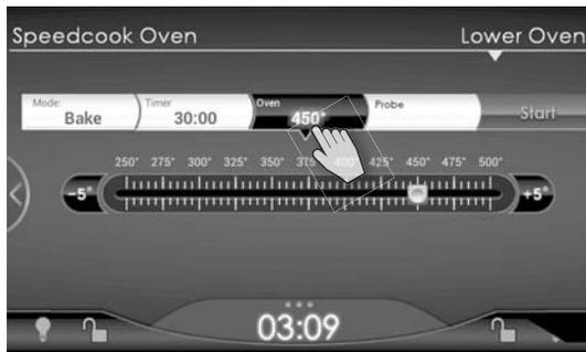
3. Slide the white button, which moves in 5° F increments to set the oven temperature.
