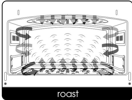
In Roast mode (see the screen in the introduction to Cook mode), the Speedcook Oven uses a combination of low and high speed air to brown the outside of food while retaining moisture inside.
