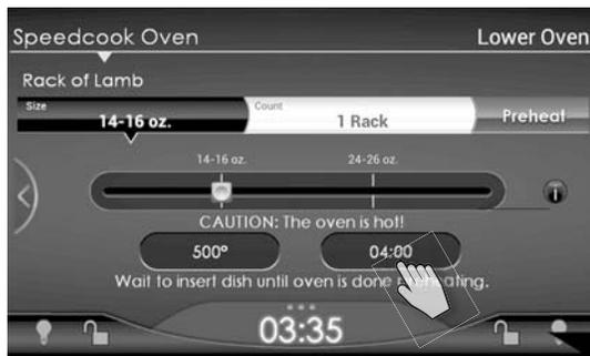
1. Tap the preset time or temperature to make any adjustments you wish to time and/or temperature as described in the preceding sections.
