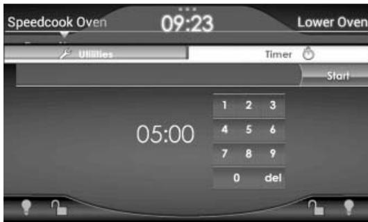
Once Start is selected, the Timer Screen closes and returns to the Main Screen. The clock at the bottom is replaced by the Timer.
