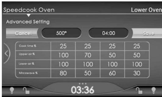
**Time:** The interval's length is a percentage of the total cook time. In the screen shown above, the total cook time is 4 minutes so each interval is 1 minute (25% of total) in length. When time intervals are adjusted, they must total 100%.
