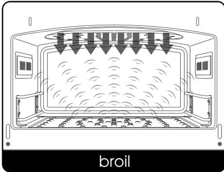
The Broil mode on your Speedcook Oven will yield the same or superior results as broiling in a traditional oven. The only difference is that your food cooks faster due to the hot air moving through the cook cavity at increased speeds.
