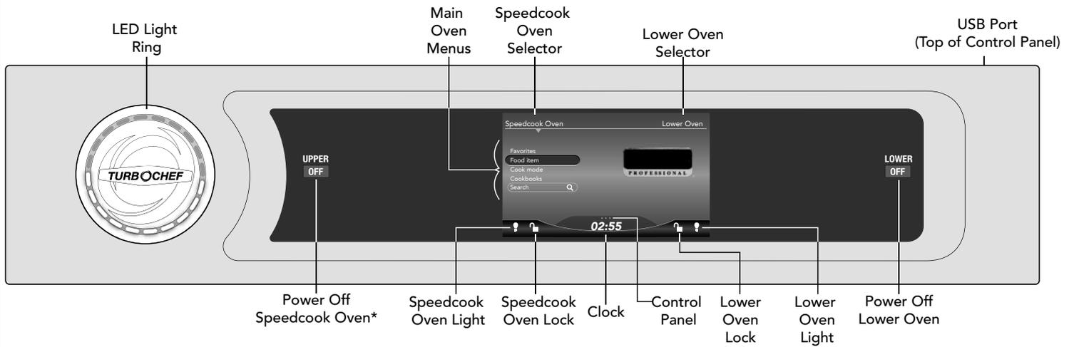
**\*Note:** Holding "Upper/Off" for more than 5 seconds will reset the oven software.
